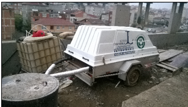
Fig.7. TRT test device of Center for Environmental Research of Cukurova University
