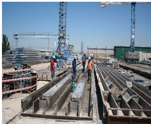
Fig.1. Precast pile at the factory Rodio-Kronsa
